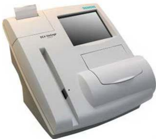
A point-of-care device used for the quantitative measurement of hemoglobin A1C in blood. Instructions for how to use the device can be found here .
